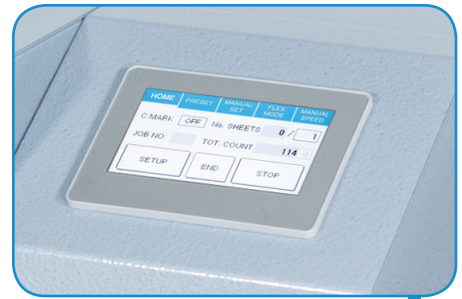
Color touchscreen control panel
